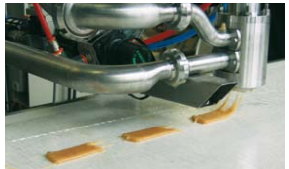
Jam topping trial: Highly viscous jam had to be laid perfectly on biscuit.
