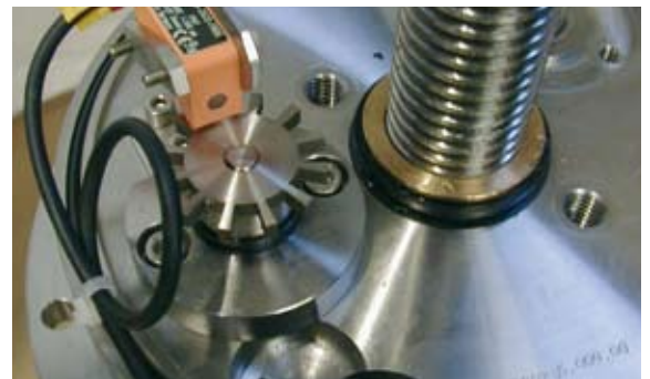
Precision dosing: Dosys™ piston pump with position sensors provides +/-0,5 % accuracy.
