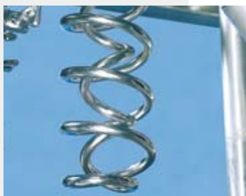
Low shear screw profile preserves product texture and flow rate.
