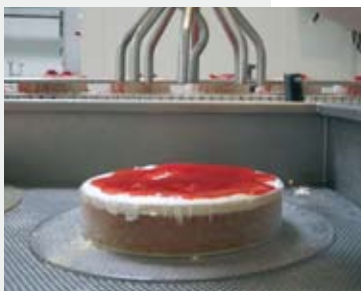
Accurate multi-nozzle dosing of fragile raspberry pastry coating.
