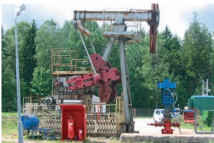
Size comparison of PCP drivehead (in blue) and typical beam pump (in red)
