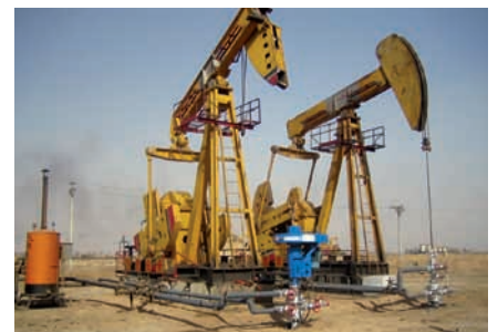
Typical beam pump replaced by PCP for production optimization
