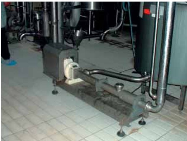
13H6: dairy industry - transfer of condensed milk to an evaporator.
