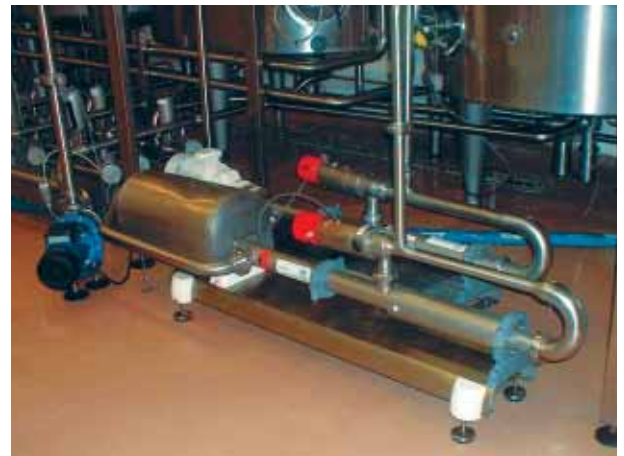
13H12: equipped with by-pass for cleaning in place in the fresh dairy product sector - dosing of cream.
