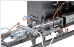
Dosys pump driven by Electro-Thrust Cylinder
