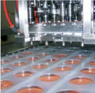
PCM dosing accuracy is +/- 0.5%
