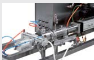
Dosys pump driven by Electro-Thrust Cylinder
