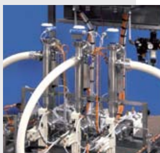
Dosys pumps and ingredients detection device
